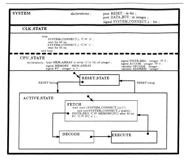
Figure 5: SYSTEM SpecChart after connections are transformed
