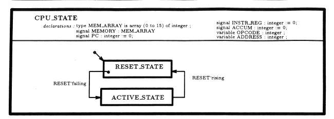
(a) CPU\_STATE with initialized signals in the declaration section
