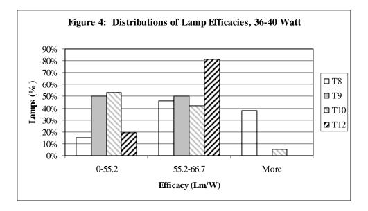
Efficacy distributions in figure 4 indicate that in the 36-40 watt category, T8 and T12 lamps have almost equally good compliance rates, while only half of T9 and T10 lamps meet the current requirements. Again, T8 lamps seem to be most efficacious of all lamp types; however, only 38% of T8 lamps have higher than average efficacy of all T8 lamps in the category.
