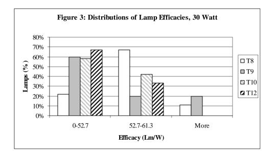
Data in figure 3 indicates that roughly 60% of T9, T10, and T12 lamps fail to meet the current performance standard, with T12's non-compliance rate the highest among all lamp types. While T8 lamps are most efficacious on average within this group, 22% of T8 lamps still fail to comply with the existing national performance standard for fluorescent lamps.
