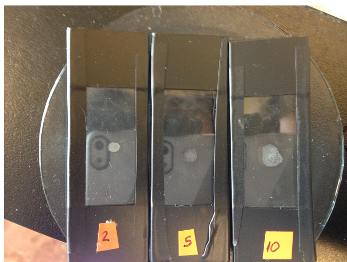
Figure 4.12: Set of Eu-DGA-SBA fluorescence samples with 2, 5, and 10 \mu\text{L} deposition of Eu-DGA-SBA in HNO 3 suspension
