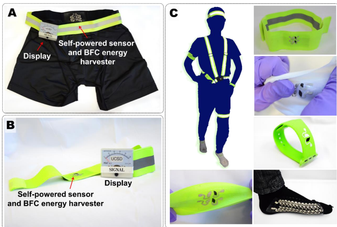
Figure 2.10 The fully integrated system for wearable lactate biosensing showing the “scavenge-sense-display” concept. The stretchable BFC arrays were printed on (A) the wearable underwear textile and (B) the stretchable strap. (C) Illustration of a ‘green’ model and photographs of wearable energy harvesting system and self-powered BFC array printed on conventional textiles and different body-worn accessories, such as stretchable headbands, straps and socks. Adapted with permission. [27] Copyright 2016, The Royal Society of Chemistry.
