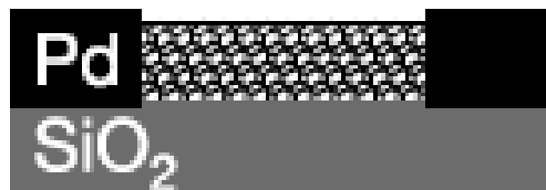
(Fig 2.4: Structure of ballistic electronic device made from carbon nanotube) [24]
