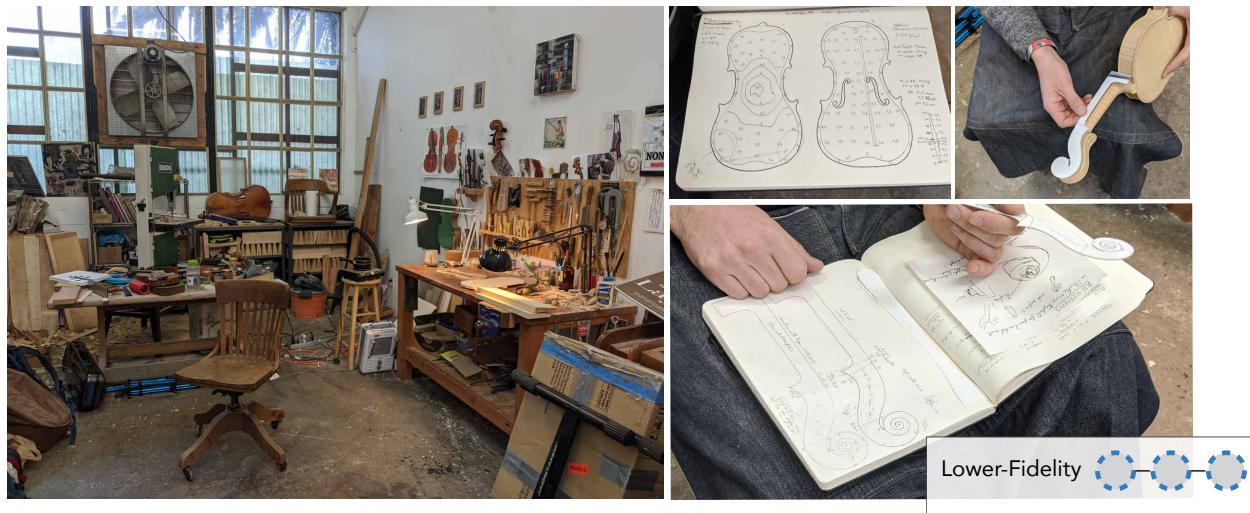
Figure 5.7: Low-fidelity records. The Violin Maker captures version histories in a variety of physical forms. From Left: The Violin Maker’s workshop. Gradation diagrams used to record the depths of the top and back of a violin. Demonstrating a paper template for carving a neck and scroll on the partly-assembled instrument. The Violin Maker’s notebook in which he records designs and modifications, showing versions of the neck template alongside the final template.
