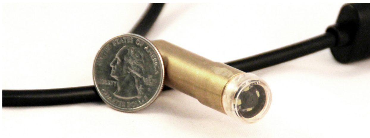
Figure 6.4: The hardware can be miniaturized, as in this pipe inspection camera with integrated LEDs.
