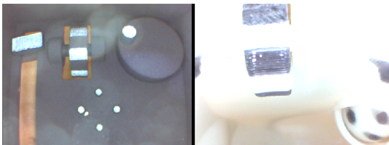
Figure 6.11: Components with reflective ink on black material (left) and black ink on white material (right).
