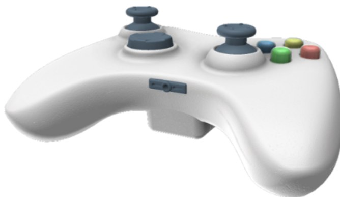
Figure 6.18: This model found online is too shallow to sense with Sauron—occlusion and curvature would prevent correct sensing with computer vision. (By user Kevin Schneider on GrabCAD, from https://grabcad.com/library/game-controller , by permission.)
