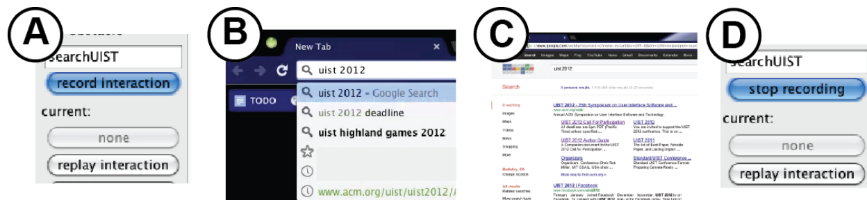
Figure 4.4: Users start to record GUI interactions in the sensor editor (A); they can for example activate the browser, enter text (B), and click on a search result (C), before concluding the recording (D). This sequence of actions can then be triggered by a touch event.
