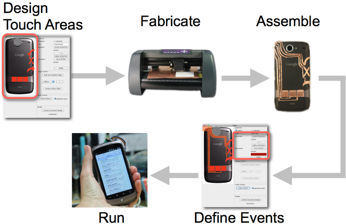
Figure 4.1: Midas enables users to define discrete and continuous touch sensors with custom shapes and layout. It generates fabrication files and assembly instructions. Designers can also define the interaction events of their prototype.
