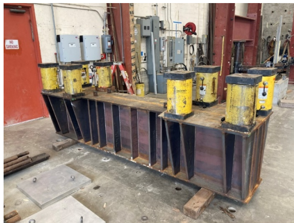
Figure 8.2 Eight hydraulic jacks (the yellow cylinders) attached to the FTSL fixture
