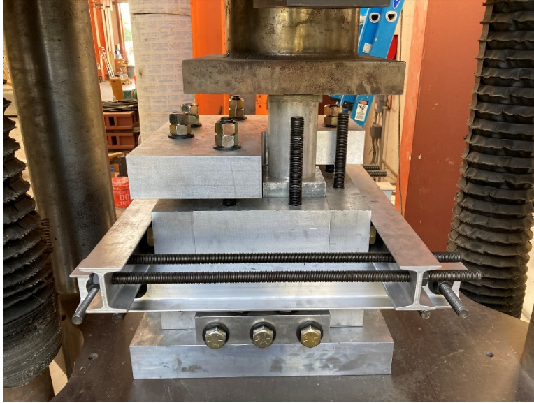
Figure 7.5 S-CSA: compacting the pistons individually through the extension rod
