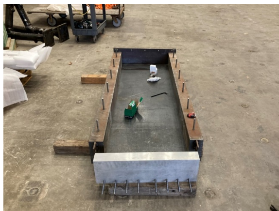
Figure 8.4 The steel mold. The compaction plates are not shown.
