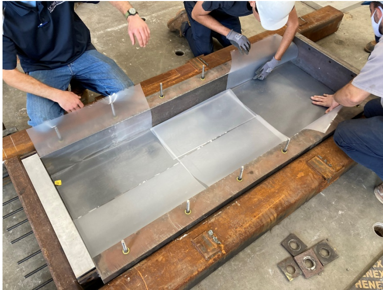
Figure 8.11 Covering the mold by a liner.
