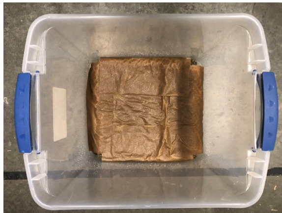
Figure 7.8 Moist curing at room temperature for 28 days
