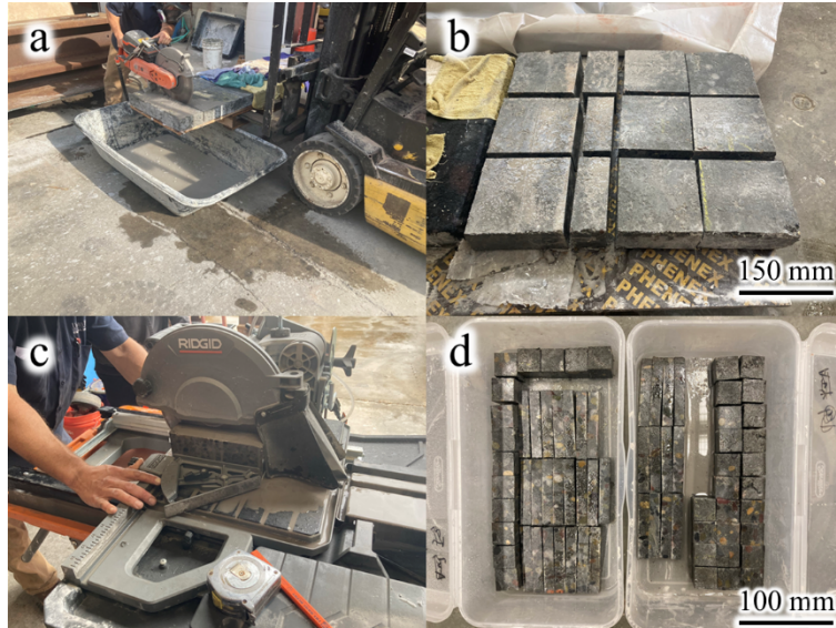
Figure 8.24 Specimen cutting: (a) dividing a slab-sized concrete sample by a Husqvarna K970 III concrete saw; (b) blocks from different locations (corner, interior, and boundary); (c) harvesting testing specimens from each block; (d) the sectioned cubic specimens and beam-shaped specimens
