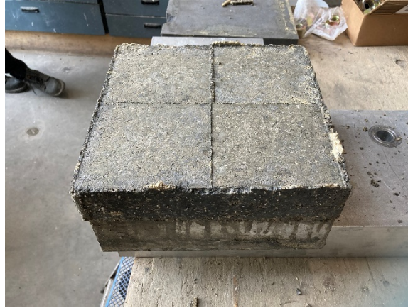
Figure 7.7 An extracted paver-sized low-binder-content green concrete sample
