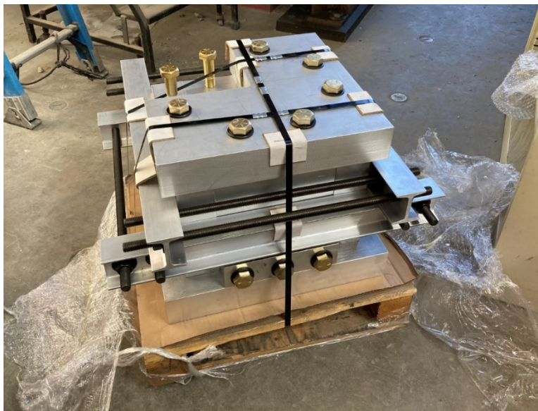
Figure 7.1 The assembled compaction system (PS20)
