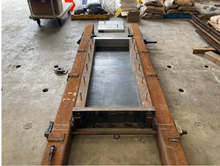
Figure 8.6 The reinforcing frame and the mold (front view)
