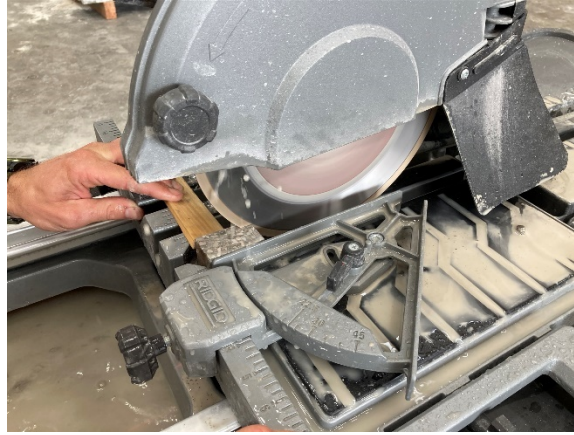
Figure 7.9 Cutting the paver-sized sample into cubic and beam-shaped specimens
