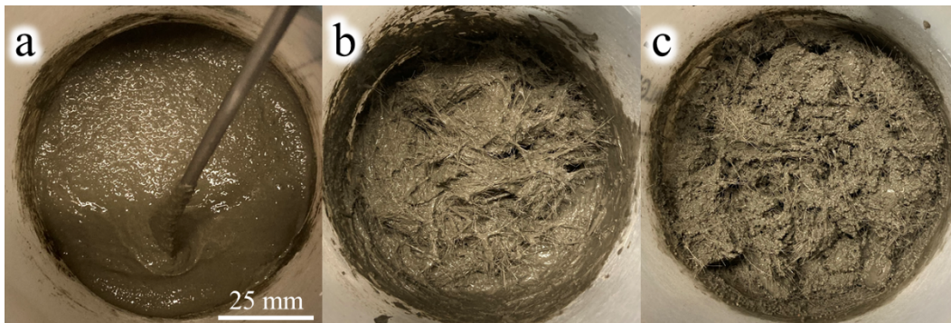
Figure 6.2 The two-step pre-mixing procedure: (a) paste formation, (b) MF dispersion, (c) and the final mixture.
