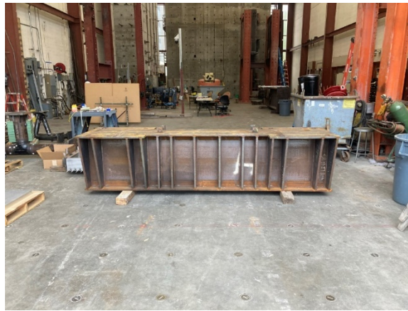
Figure 8.1 The 3.3 m-long flexural test steel load (FTSL) fixture.
