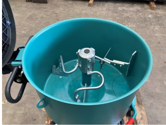
Figure 8.13 The chamber of the Collomix TMX 1500 mixer
