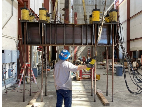
Figure 8.3 The hydraulic jacks are attached to the reinforced concrete floor.
