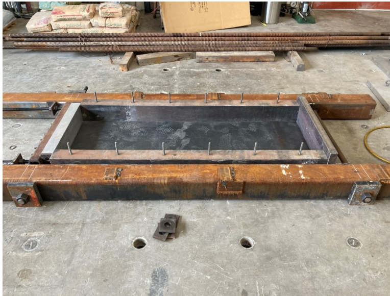
Figure 8.5 The reinforcing frame and the mold (side view)
