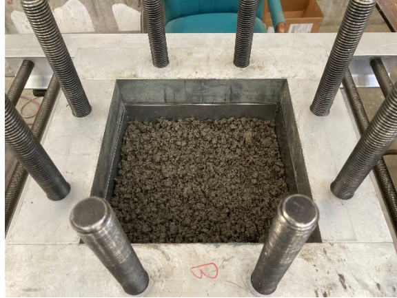
Figure 7.3 Transferring the pre-mixed materials into the PS20 mold.
