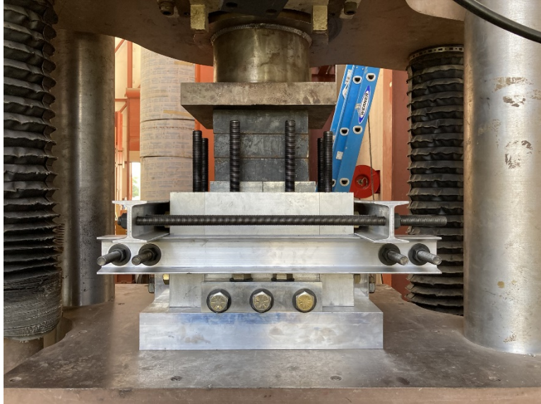
Figure 7.4 Initial compaction: compacting the four pistons simultaneously
