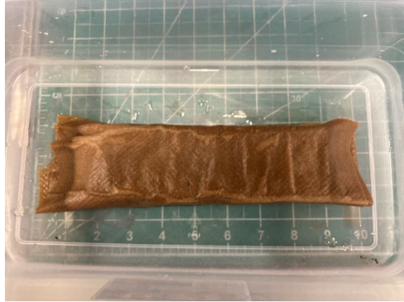
Figure 6.5 Moist curing for 28 days
