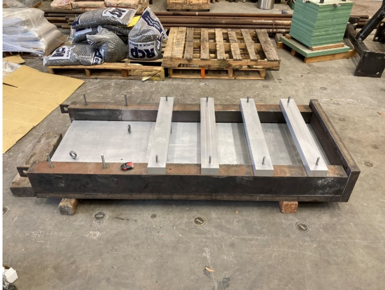
Figure 8.8 The compaction plates and the fixing bars
