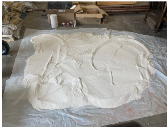
Figure 8.9 Sand drying for 2 days
