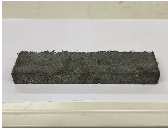
Figure 6.4 A sample removed from the compaction system after initial hardening for 2 days
