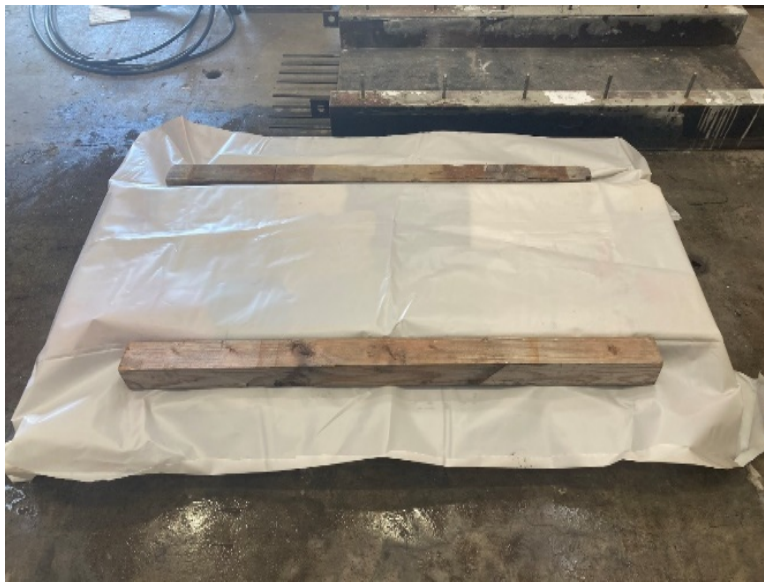
Figure 8.23 Moist curing at ambient temperature for 28 days
