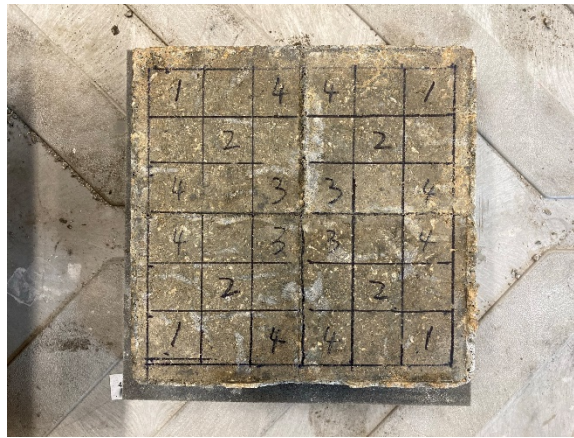
Figure 7.10 Harvesting specimens from different locations of each sample
