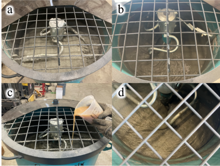
Figure 8.15 The first step of pre-mixing: (a) mixing of dry materials, (b) adding water into the mixer, (c) adding VMA, and (d) the produced paste.
