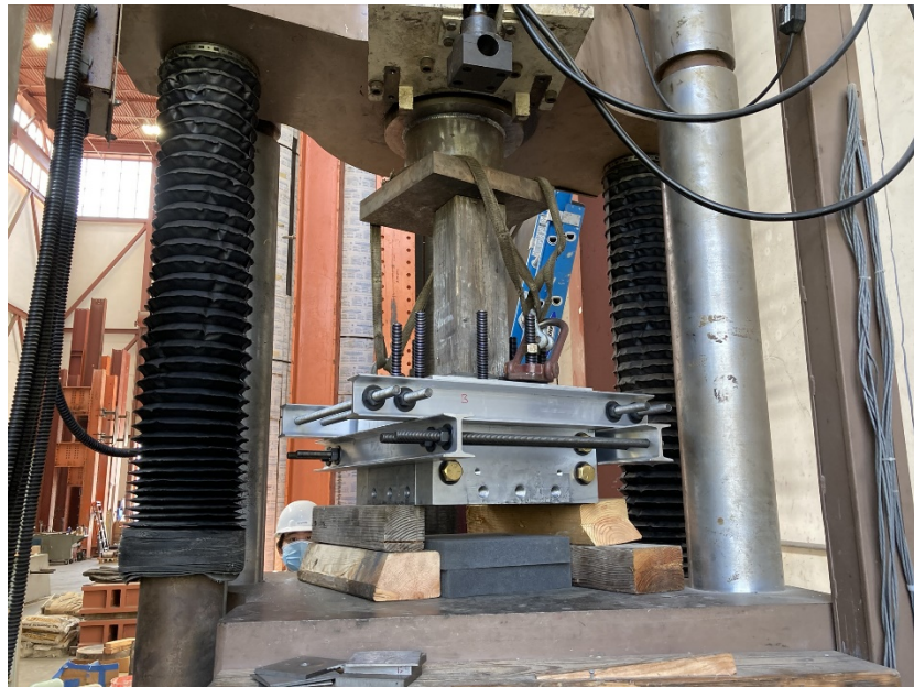
Figure 7.6 Removing the bottom plate and pushing the sample from the bottom opening of the PS20 mold.
