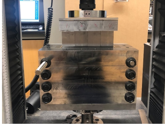
Figure 6.3 Compressing the four compaction pistons simultaneously
