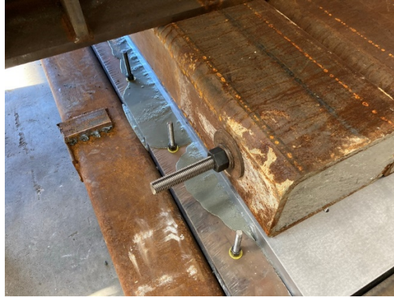
Figure 8.28 Binder loss of Sample 1 during compaction
