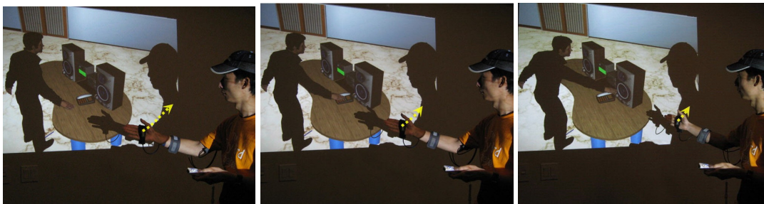
Figure 5.3: Our interface allows the user to easily scroll through captured motions, crop out unwanted frames, and most importantly mark stroke frames to be parameterized. This image shows the user inspecting one motion segment controlled by hand movement.
