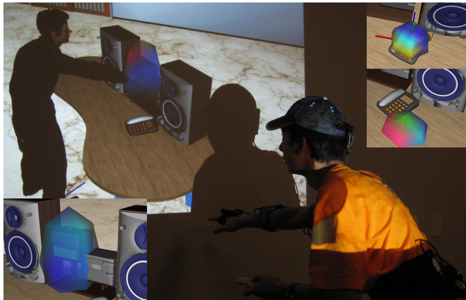
Figure 5.5: Local Coverage Visualization mode. The rendered surface follows the movement of user's hand, ideal for checking small ROIs like dials and buttons.
