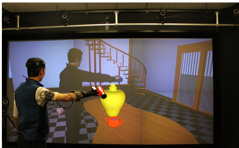
Figure 5.2: Example scenario (parameterized water pouring motions) of our motion modeling phase running on the UC Merced PowerWall system. Motions are captured on-line with GestureVest .
