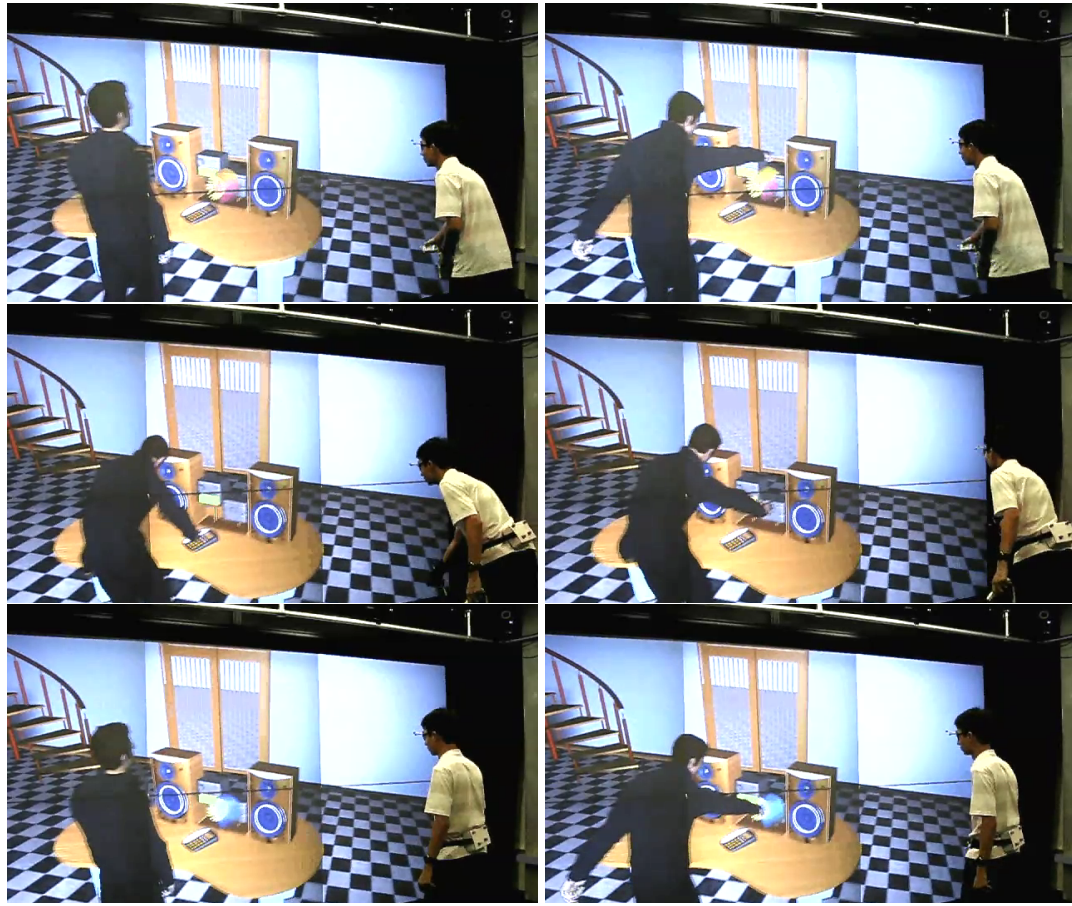
Figure 5.7: The sequence demonstrates the process of on-line modeling and dataset refining. Top row: user spotted ROI with low coverage, note the red color shown by the LCV tool. Middle row: user teaches agent new motions towards the low coverage region via direct demonstration; Bottom row: coverage is improved for this ROI, as a result the agent could better synthesize pointing motions towards this ROI. Note the color shown by the LCV tool turned into blue, indicating improved local coverage.
