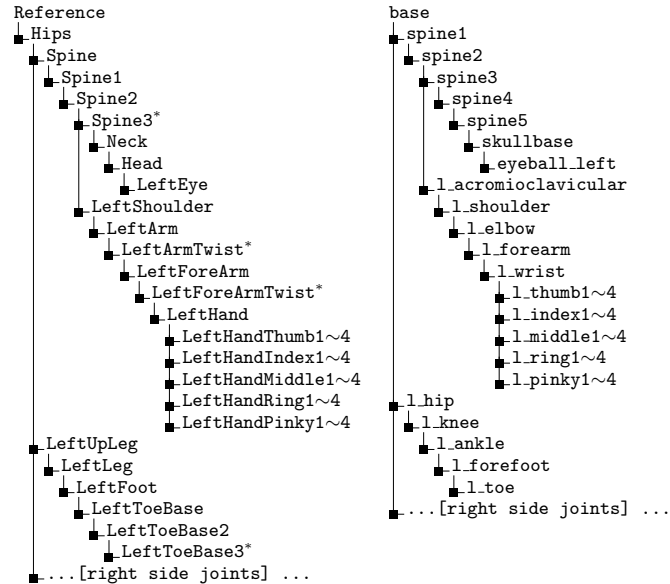
Figure 8.2: Final mapping result achieved by SmartBody, left side is given as an example following MotionBuilder naming convention, right side is the corresponding joint names in SmartBody. * denotes joint (if exists) is skipped as it's not handled by SmartBody.
