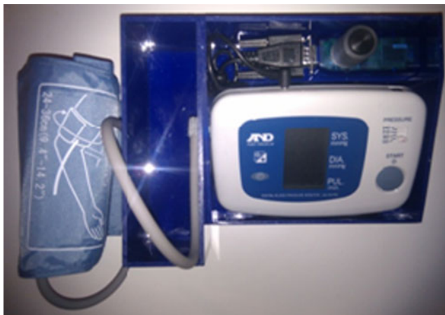
Fig. 5 Designed Bluetooth-enabled blood pressure monitor
