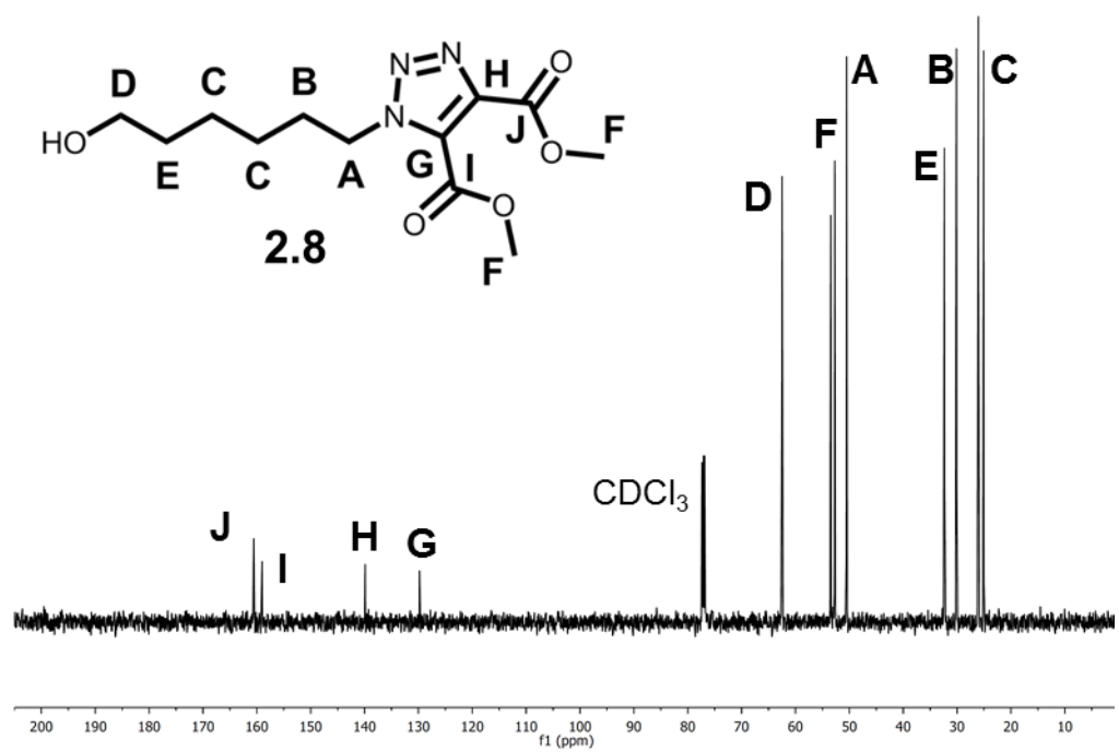
Figure 2.14 ^{13}\text{C-NMR} Comparing 6-Azidohexan-1-ol ( 2.7 , Top) and TRZ-DiMe Hexanol ( 2.8 , Bottom)
