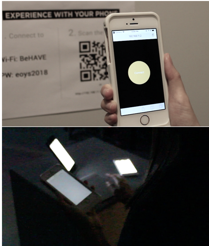
Figure 4.13: Audience interaction. After accessing the mobile web page via a QR code or a URL with their mobile phone, the audience can see the user interface to connect or disconnect to the BeHAVE main web (top). The screens of the connected mobile phones are flickering (bottom).
