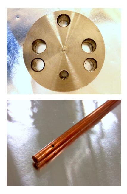
The electrodes are machined from 1/8" OD copper rods with ~10" length. We have found the 1/8" OD copper rods ordered from Mcmaster-Carr may not always fit the 1/8" ID alumina tube, 3 mm OD copper rods can be used as an alternative. Each electrode has a 1-72, 1/4" depth tapped hole at one end. A side hole with ~0.03" clearance need to be drilled at the bottom of the tapped hole to pass through the tungsten filament. The actual diameter of this side hole may depend on the filament thickness.
