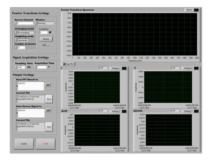
modes, the program will conduct several runs of measurements base on the "number of passes" and average them. The "completed" box displays the current pass number. The green indicator will light up when all the passes are completed. The "dB" switch specifies whether the results are expressed in decibels.
