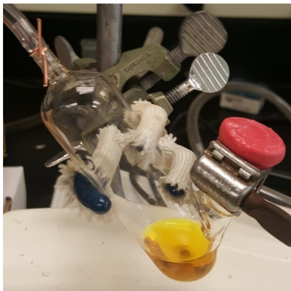
Figure 3.S4. Pressure testing vessel (total volume ~48 mL).
