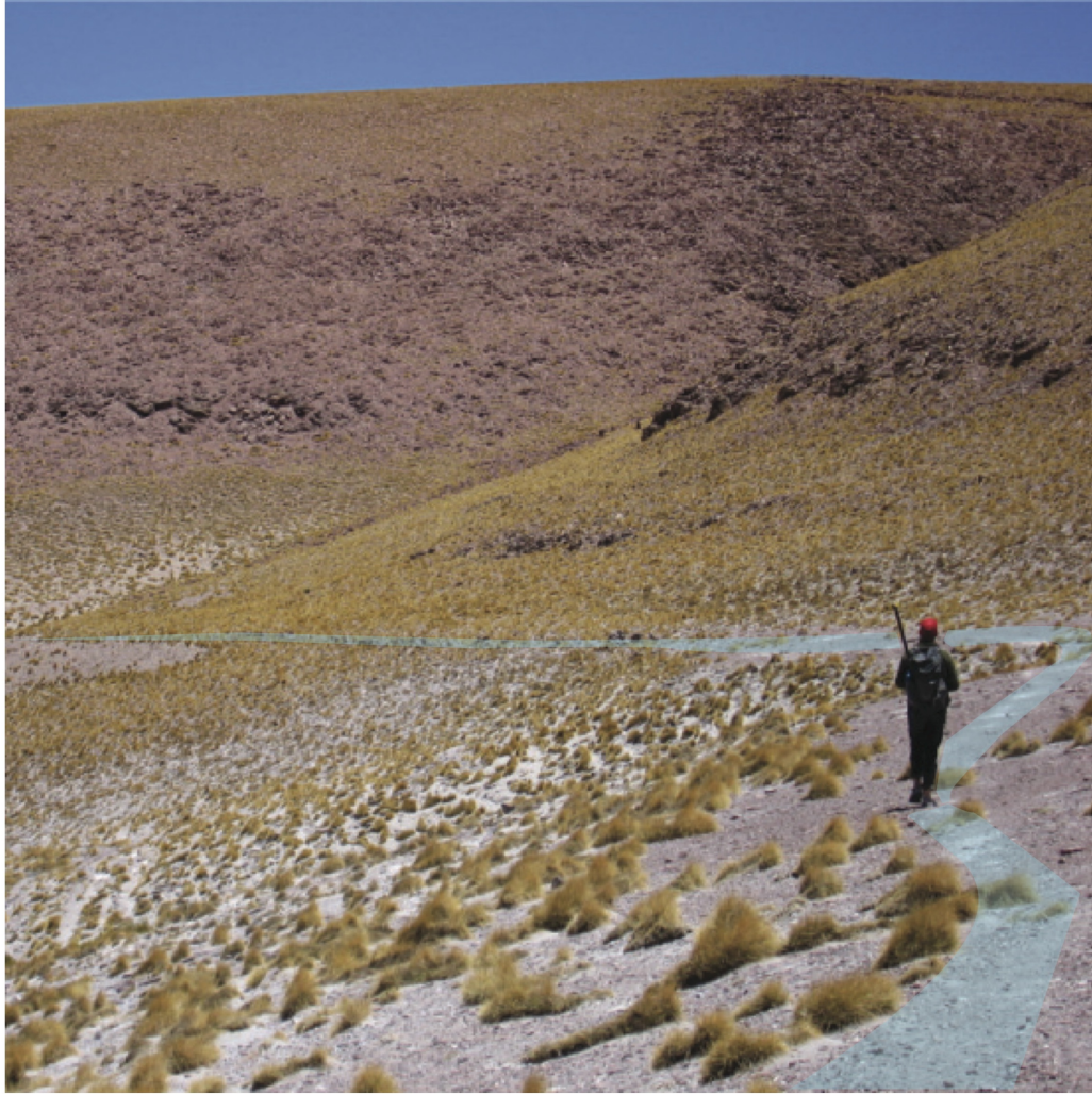
Figure 3.5: Photo looking to the east along the southern shore of Laguna Mama Khumu. A prominent strandline is highlighted in translucent blue. To survey shoreline elevations at Mama Khumu, we walked along them with a kinematic differential GPS receiver mounted on a pole in a backpack. Though in this image the pole is slightly askew, vertical uncertainties in elevation are on the order of 50 cm with this method.
