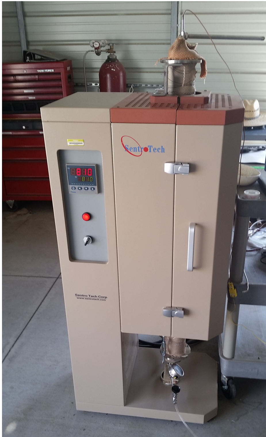
Figure 6.2: Biochar activation experimental setup.
