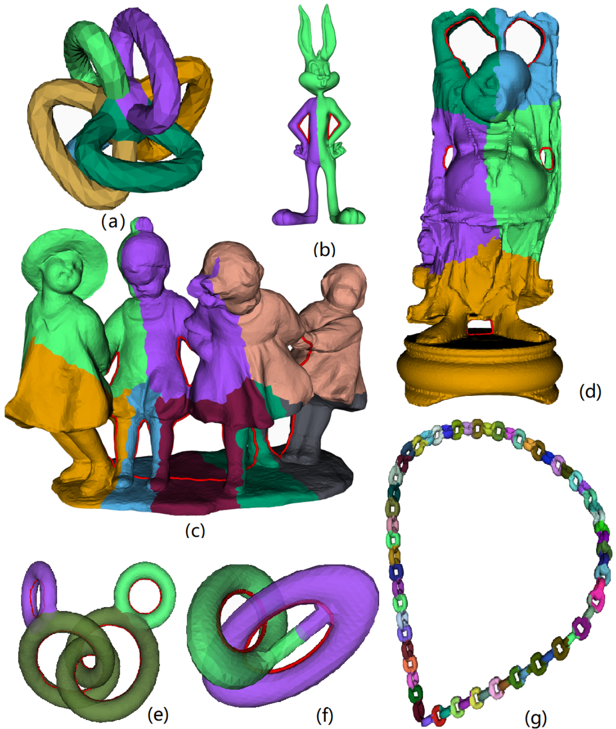
Figure 4.11: Tori decomposition results of our method, with tunnel cycles highlighted in (b)-(f). One of the tunnels in (e) is knotted and (f) contains tunnels interlocking with each other. (g) has genus 64.
