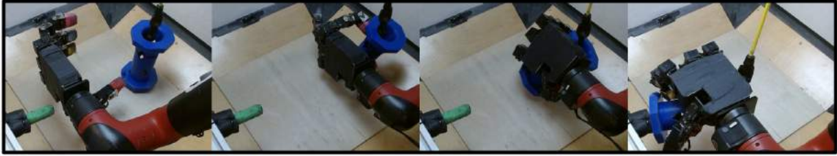
Figure 33: Filmstrip of final learned insertion behavior. Using the user-provided milestones, our robot learns a set of skills (e.g., grasp, insert), which together specify a long horizon task as well as the stages needed to practice autonomously. In our experiment, the robot learns to successfully plug-in a hose connector over 36 hours of continuous learning without instrumentation, purely from image observations and joint encoders.
