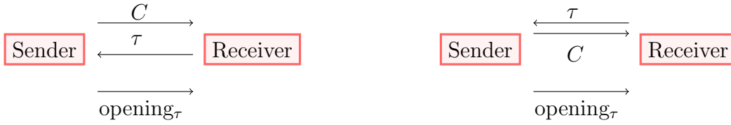
Figure 1.1: The diagram on the left depicts the communication pattern of Khurana’s [Khu21] commitment scheme, whereas the diagram on the right depicts ours. The key difference is that in our scheme, the receiver’s message and the sender’s messages can be sent simultaneously, while in [Khu21] the receiver’s message must be sent after the sender’s message.
