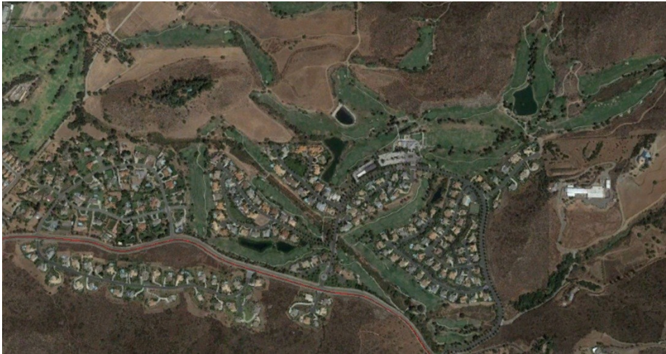
Figure 2.1 Example of clustered development with a golf course buffer between the development and the wildland vegetation in San Diego County. Image courtesy of Google Earth.
