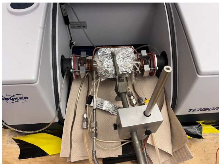
Figure 2-2. Picture of Transmission cell covered with heating tape used in this dissertation.
