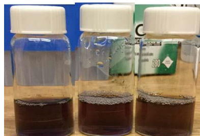
Figure 3.5 AuNR with CTAB increase from left to right
