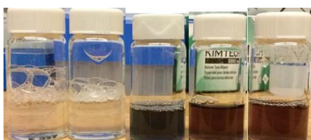
Figure 3.10 Gold nanorod growth with different kinds of seeds
