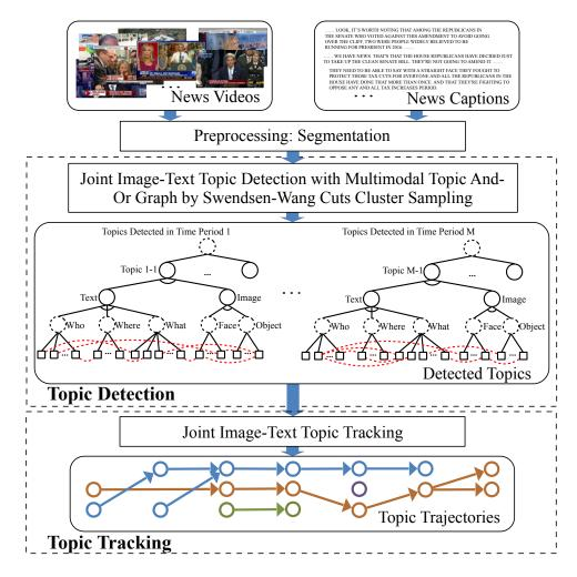
Figure 3.1: Overview of the proposed topic detection and tracking method. The inputs include both news videos and closed captions (texts). We detect topics through a joint image-text cluster sampling method within each time window. Then detected topics are tracked over time to form topic trajectories.
