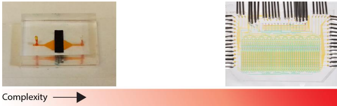
Figure 0.5. Complexity of Microfluidic Chip Design Depends on Desired Experimental Output. Simple microfluidic designs (left) do not equate to less information in comparison to complicated designs (right). Rather, the complication level of each design depends on the required information from the experiment whether it be spatio-temporal dynamics of wound response (left) or cellular response to dynamic, temporal inputs (right, image courtesy of Savas Tay at the Institute for Molecular Engineering at the University of Chicago).
