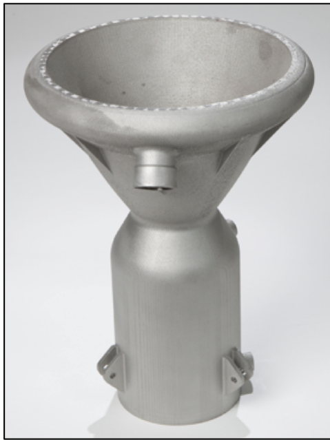
(a) SLM aerospace engine component[34]. (b) SLM skull implant for facial reconstruction[16].
