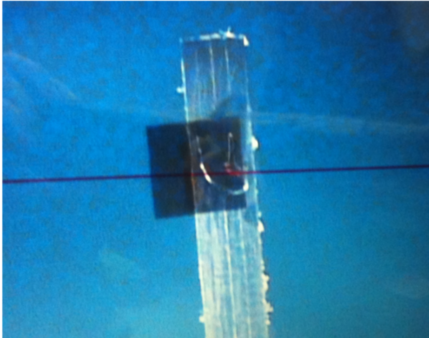
Figure 3.18: Image from the point of view of the side-lighter target. The main foil target can be barely seen through the super-fine mesh in front. Beam and target alignment must be extremely precise or else the plastic leading edge from the main target canll block the surface of the foil target.
