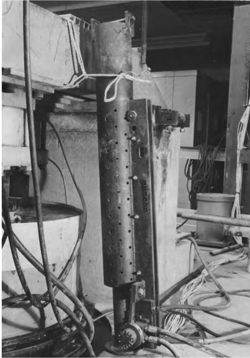
Figure A-4: Hydraulically Driven 140-lb Trip Hammer Used in WES Study (from Bieganousky et al., 1976)
