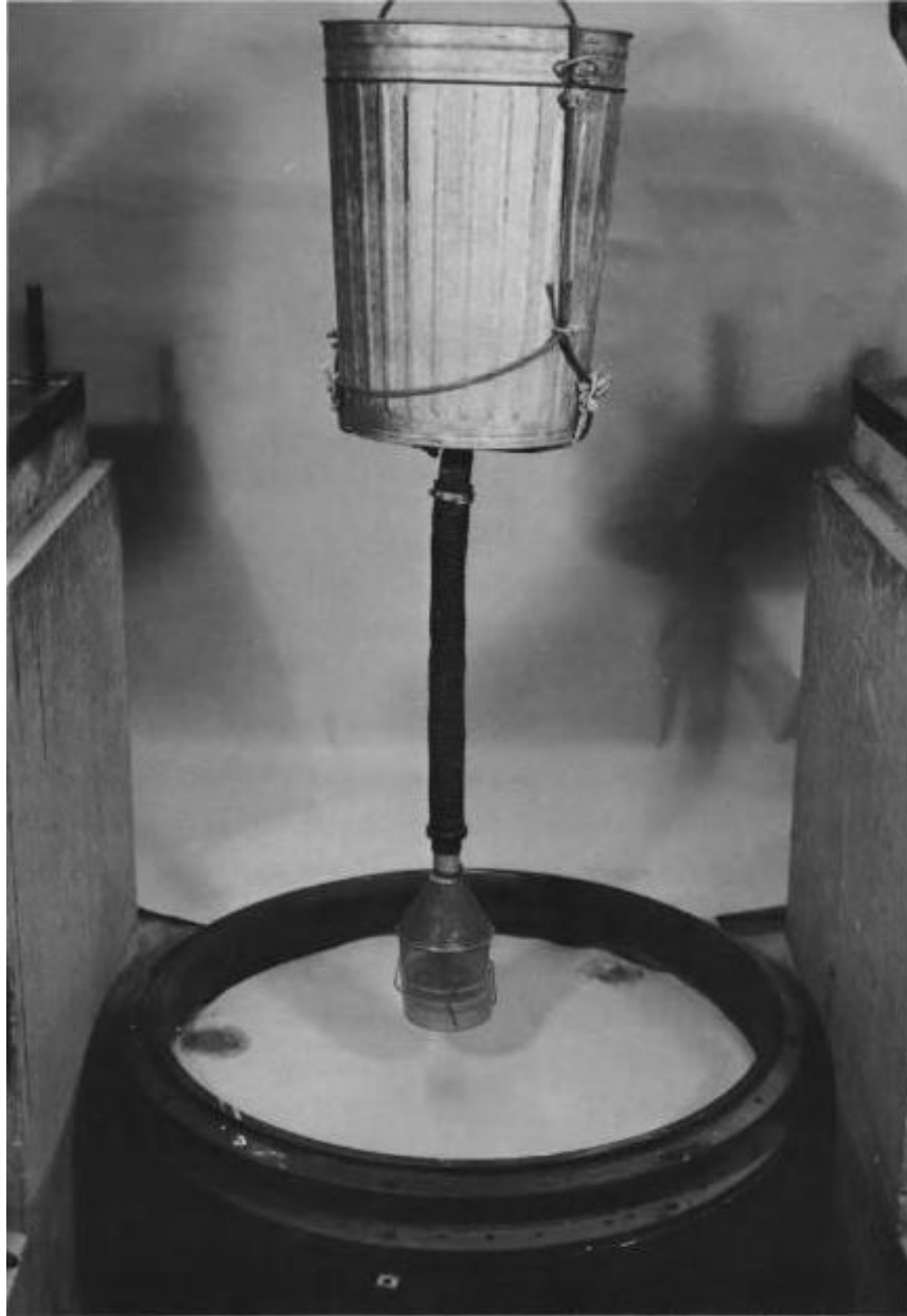
Figure A-6: Single-Hose Rainer Used in WES Study (from Bieganousky et al., 1976)
