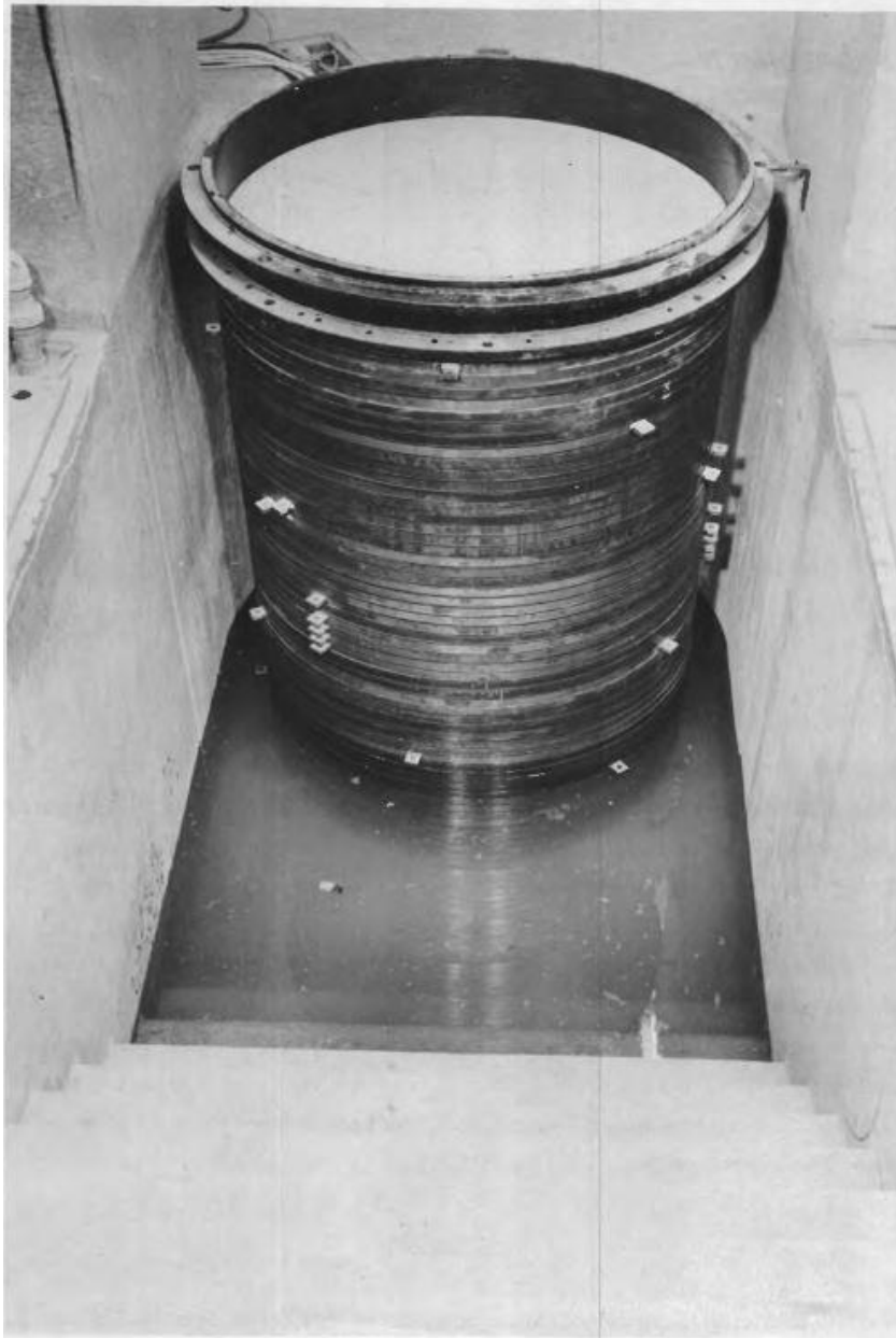
Figure A-1: Stacked-Ring Chamber used in WES Study (from Bieganousky et al., 1976)
