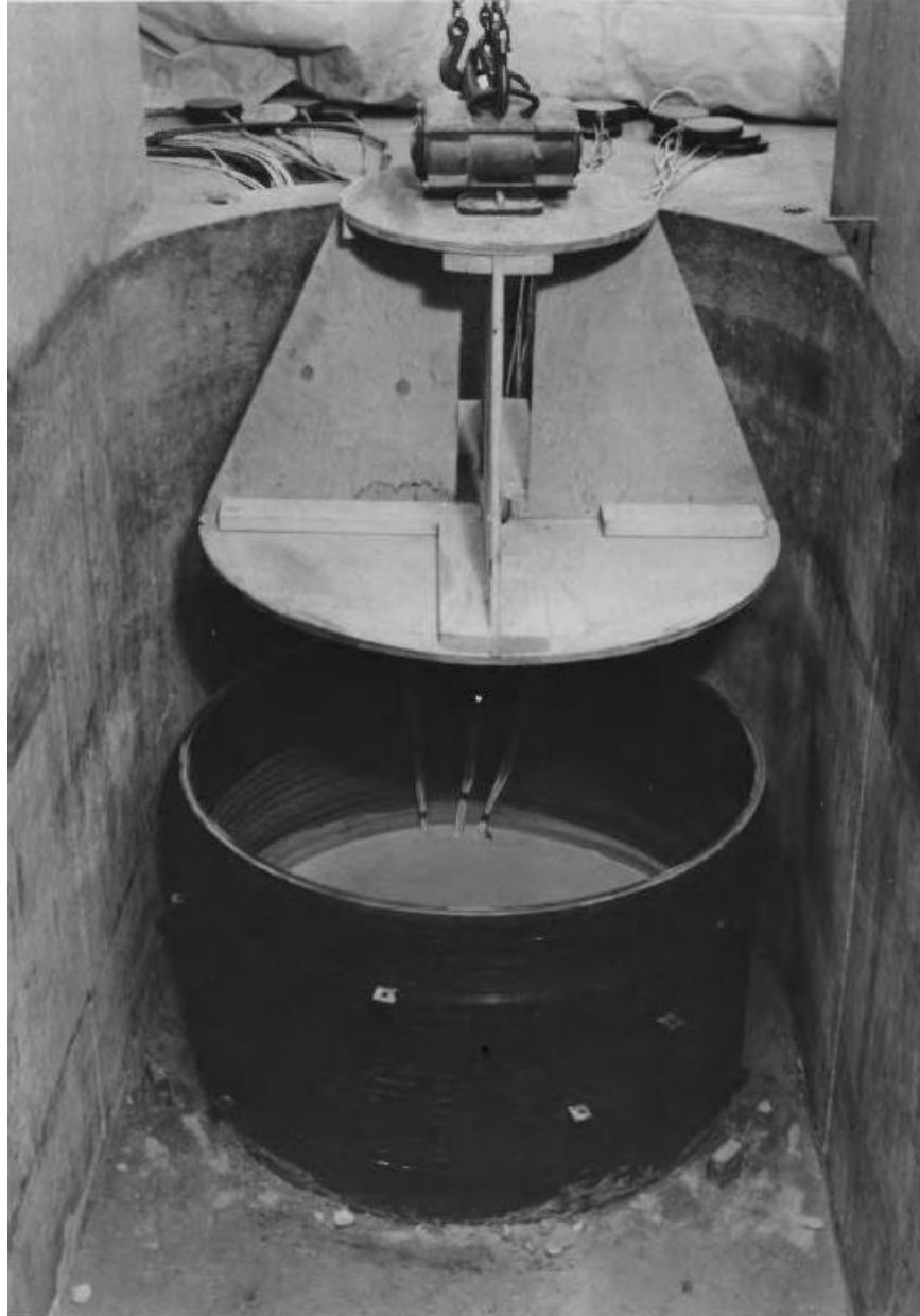
Figure A-7: Vibratory Compactor Used in WES Study (from Bieganousky et al., 1976)
