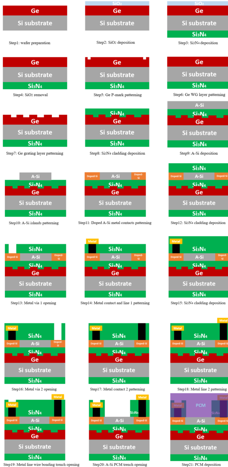
Figure 19. Fabrication process flow of the PCM-MWIR beam steering devices
