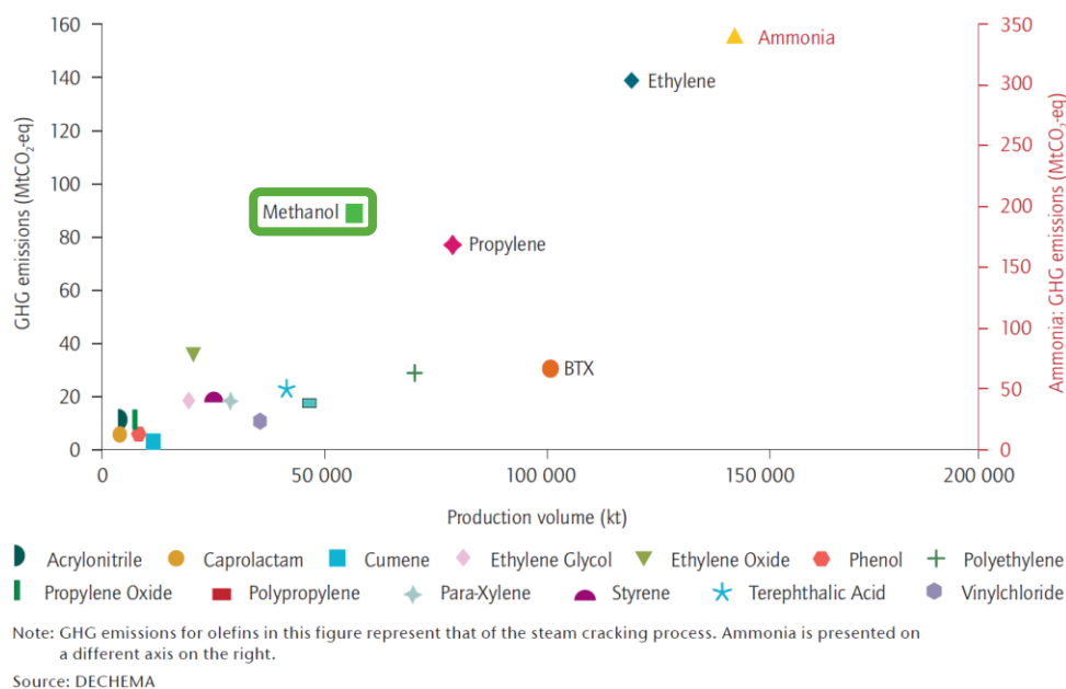
Figure 7: Greenhouse gas emissions and production volumes for top 18 large volume chemicals. Based on IEA graph from Technology Roadmap: Energy and GHG Reductions in the Chemical Industry via Catalytic Processes© IEA 2013, IEA Publishing; modified by Dayton T. Horvath. License: http://www.iea.org/t&c/termsandconditions/
