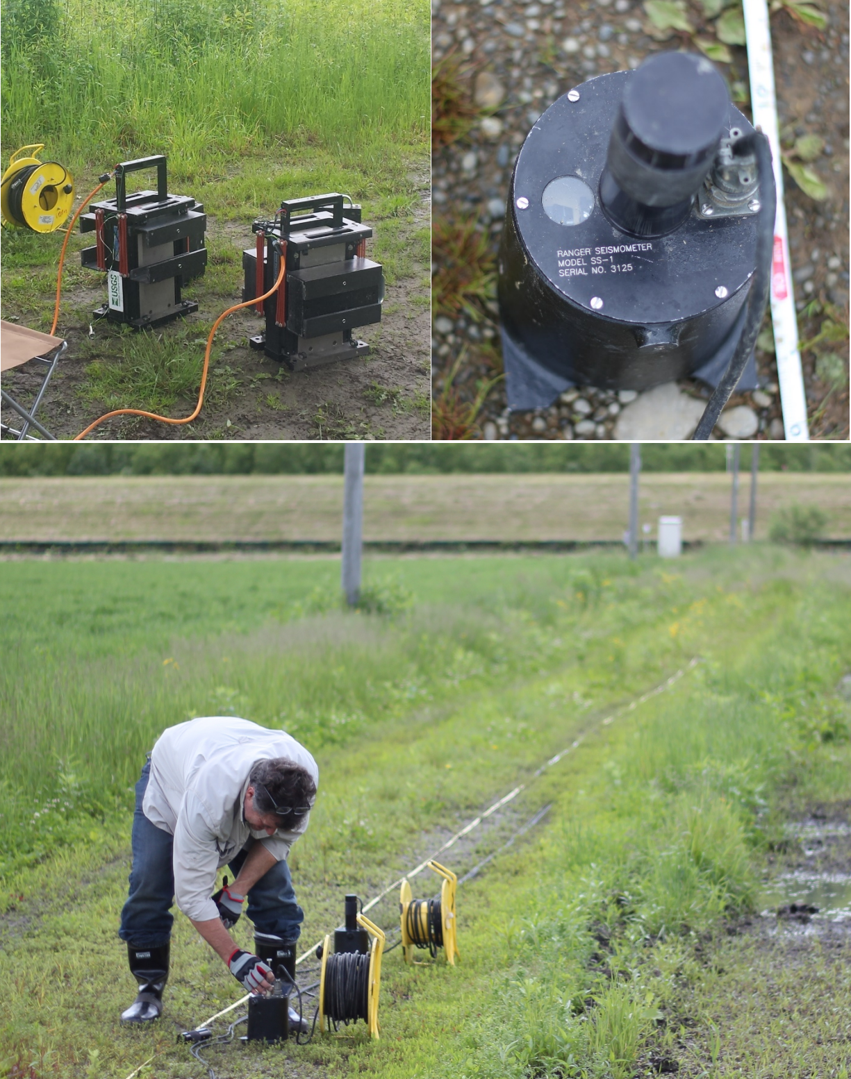
Figure 3.4 The mass shakers for generating harmonic stepped waves (top left) and the seismometer (top right). The spacing between the seismometers are changed after each sweep by the mass shakers (bottom).
