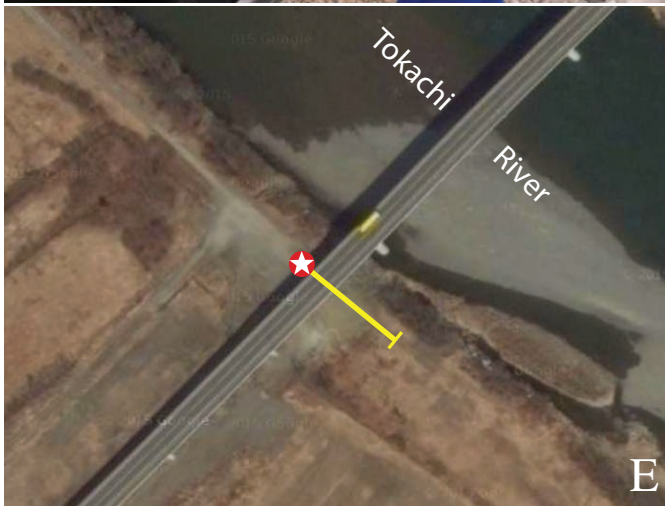
Surface wave test site 1047HK located on the SW bank of the Tokachi River 16 km east of Obihiro, Hokkaido, Japan (lat 42.92140, long 143.3858). A) view northwest from the shaker; B) view southeast toward the seismometer array; C) site information; D) view to the northeast from the test site; E) satellite view of the local site, yellow bar is seismometer array; F) site location near Obihiro, Hokkaido, Japan.
