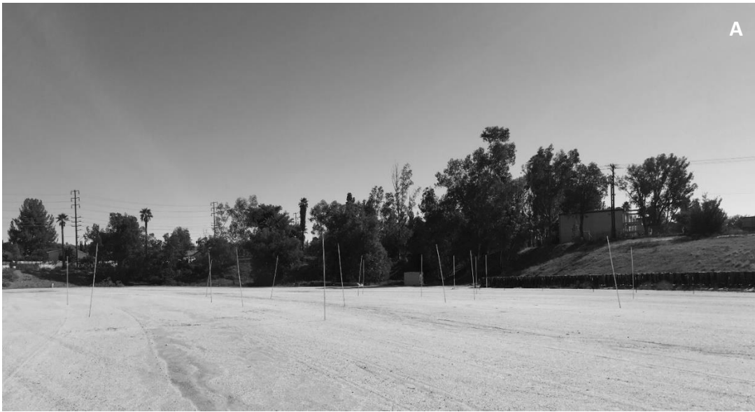
Figure 3.3: Arrangement of PVC poles covered in tangle trap. This method of recapture was a cheap but effective method for collecting house flies in flight. A) Ground level looking southeast, and B) photo taken from adjacent hill looking east, subject (5'10" tall) is standing at the fly release point in the center of the trap circles.
