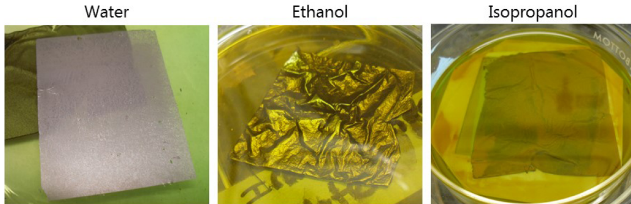
Figure 5.16 | The solvent effect on the transfer of support layer-less FLG: a. Etching of FLG-Ni in \text{FeCl}_3 and water. b. Etching of FLG-Ni in \text{FeCl}_3 and ethanol. c. Etching of FLG-Ni in \text{FeCl}_3 and isopropanol.
