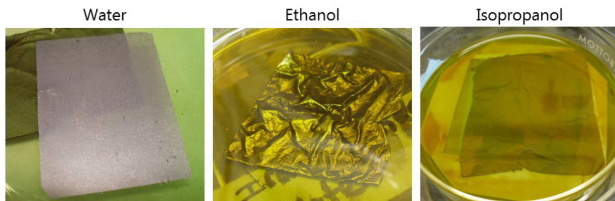
Figure 3.4 | The effect of lowered surface tension in the water-based etchant on the transfer of graphene. Going from left to right, the surface tension of the solvent decreases.
