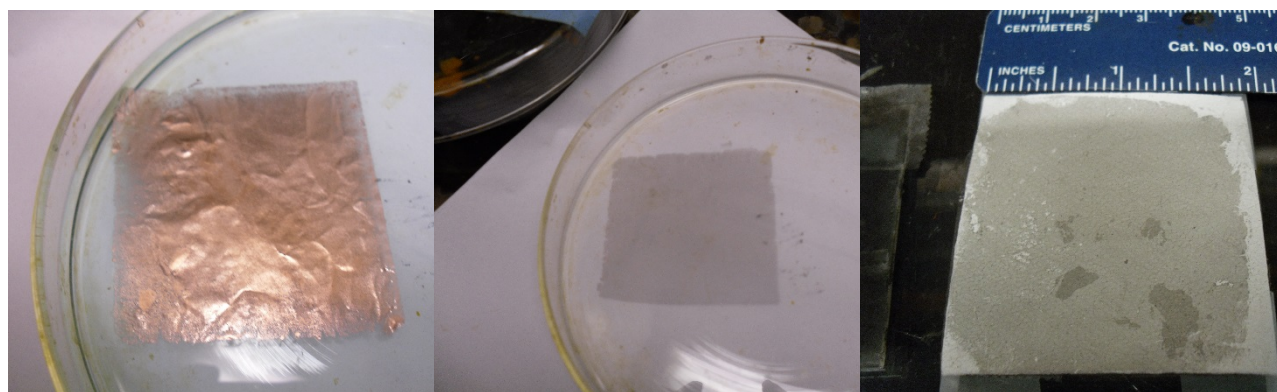
Figure 5.17 | Transfer of FLG grown Cu-Ni alloy: a. Etching of Cu-Ni alloy in APS. As the Cu etches, the solution becomes blue b. The resulting etched film is self-supported in water. c. Transferred film onto PTFE. There are noticeable tears caused by the transfer process. The extra dark regions on the transferred sample correspond to flakes that were floating in solution, but got trapped beneath the transferred sheet and the membrane support.
