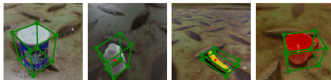
(c) Examples images from the YCB-Objects in-distribution test set shown with keypoint annotations. Each image is annotated with nine keypoints corresponding to the corners of the 3D bounding box and the object center. Models in the testbed predict these keypoints, and the object's 6D pose is recovered from keypoints using the PnP algorithm [134].
