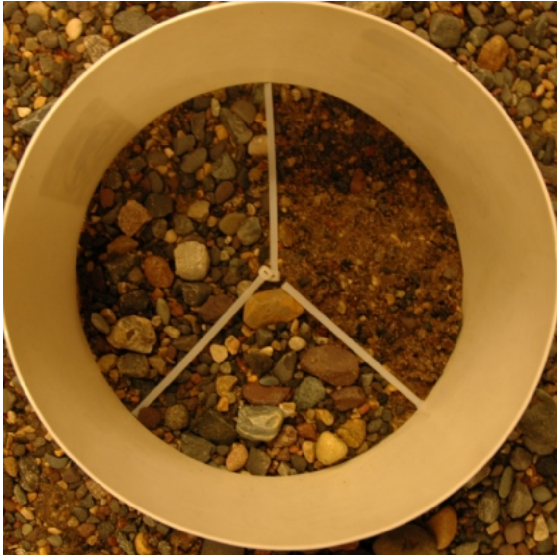
Figure 3.7: A sample pit with the surface layer removed from the upper right subsample. The other sections show the surface armor layer. The zip ties in the middle mark the borders between the three subsamples. The ring (made from a 5-gallon bucket) is pressed into the bed while excavating to prevent the walls from collapsing.
