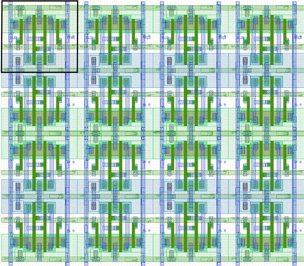
Figure 16: Layout of a 4x4 bitcell array.
