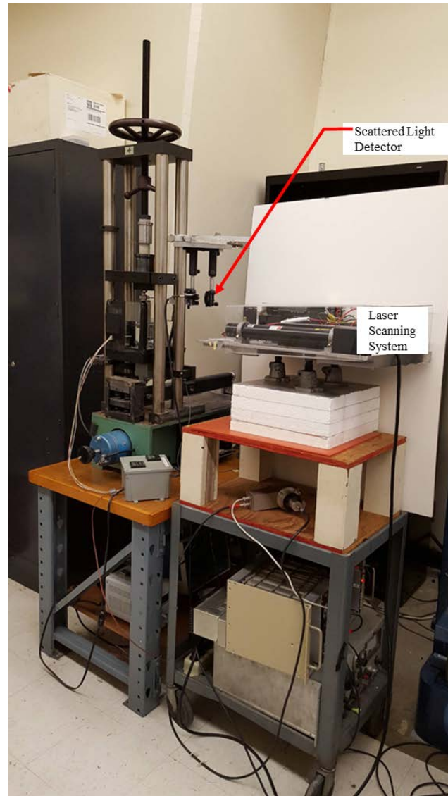
Figure 24: Laser Scanning System integrated to the setup to monitor the induced strain in the sling during the fatigue tests
