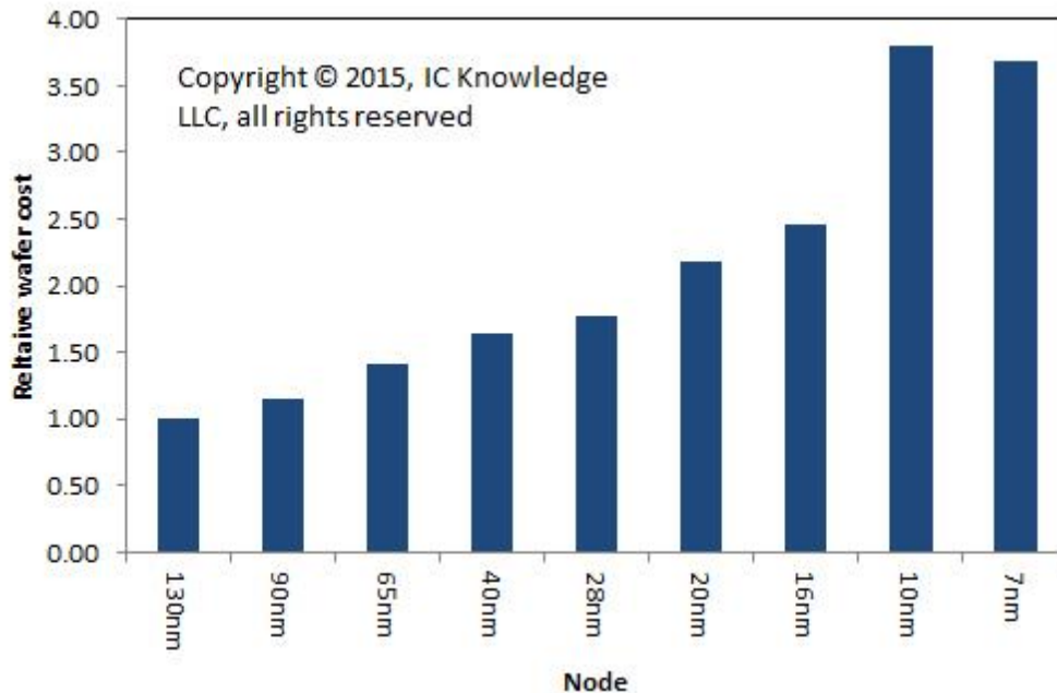
Fig. 5.1 Foundry Wafer Cost Trend. Source: IC Knowledge Cost Model [5.3]. Note: assumptions for 7 nm node are made that EUV is available and EUV has the potential to decrease the wafer cost versus 10 nm node.
