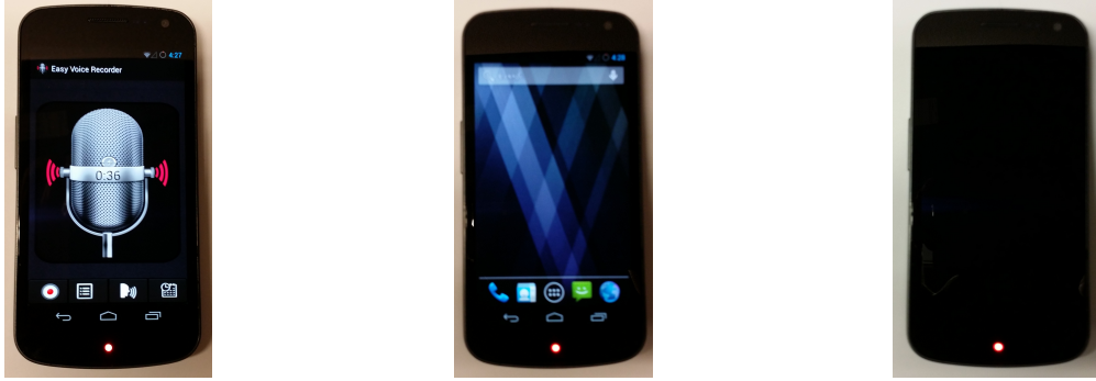
Figure 4.1: LED notification for microphone using Viola. The LED blinks even if the application is in the background or if the display is off. Malicious attempts to break this notification will be blocked.
