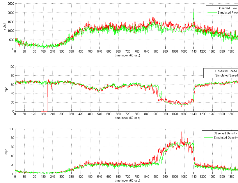
b. Modified METANET simulation output and actual BHL measurements
