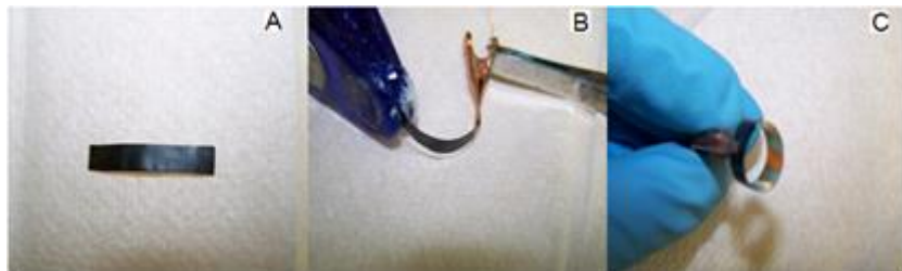
Figure 5.5 Pictures show flexibility of a copolymer unimorph actuator
