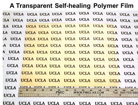
Figure 4.7 Optical photograph of a transparent MDPB-FGEEDR copolymer film (12 cm × 10 cm; the square area in light yellow color)
