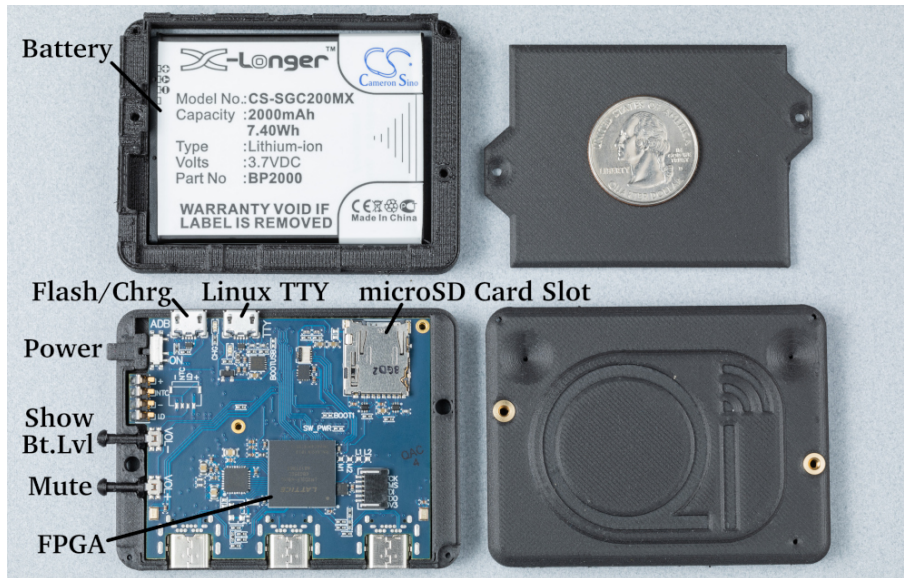
Figure 1.4. The OSP PCD disassembled, showing the battery, the back of the carrier board, and the plastic shell.
