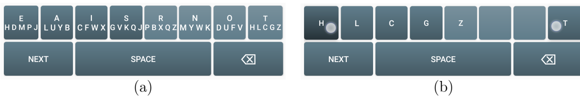
Figure 5.3: The Seniorita chorded keyboard used in the experiment. It enables users to enter text by pressing two keys simultaneously using the thumbs. (b) Pressing a key highlights all available chords for the key.
