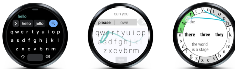
Figure 3.2: Existing text entry methods for smartwatches. The user enters the text using miniature versions of the standard QWERTY such as (a) default QWERTY method, where to enter text, the user needs to tap on the desired key or perform gesture to enter word, (b) WatchWriter, where the user can enter text either by touch or gesture typing, and a novel keyboard called (c) SwipeRing, which arranges the QWERTY layout around the bezel where the user enters text by gesture typing.
