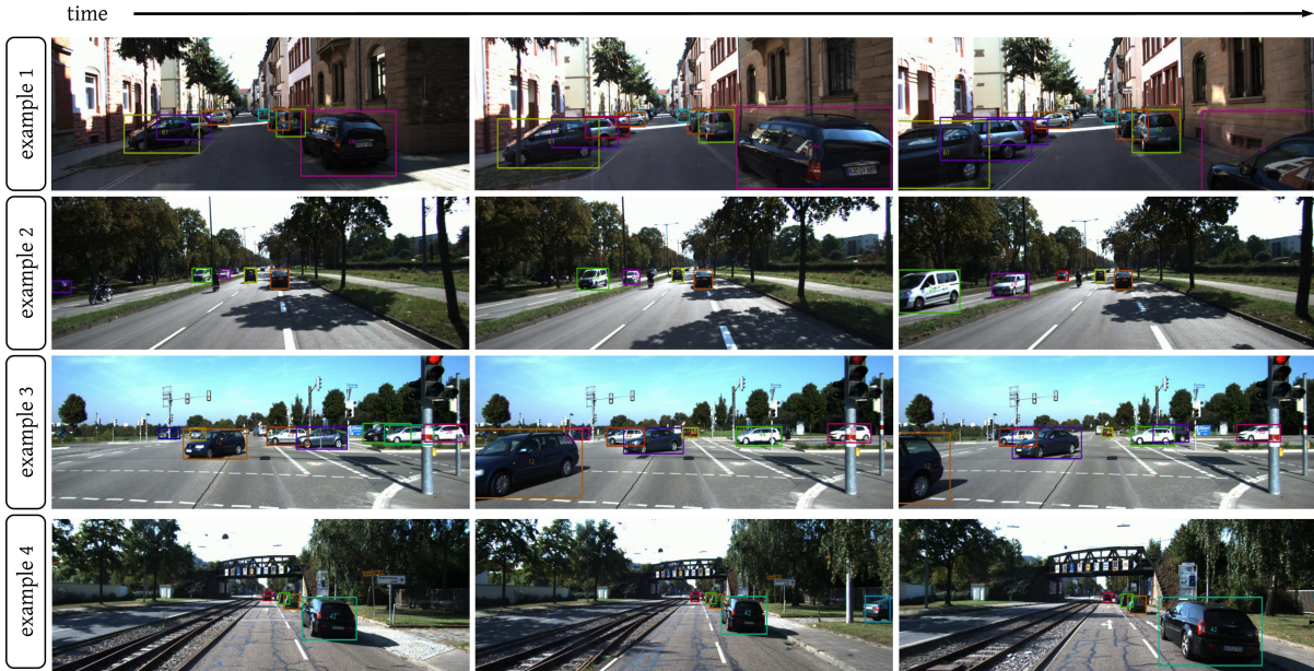
Figure 4.6: Qualitative examples on the KITTI multi-object tracking (MOT) testing set. Each row depicts a sequence of frames, with overlaid color-coded detection boxes. Each color represents a unique track generated by our model.
