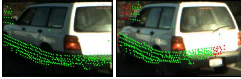
Figure A.4: Fusion of object proposals using LiDAR point clouds: Points common to both detections are drawn in green, and the rest are drawn red.
