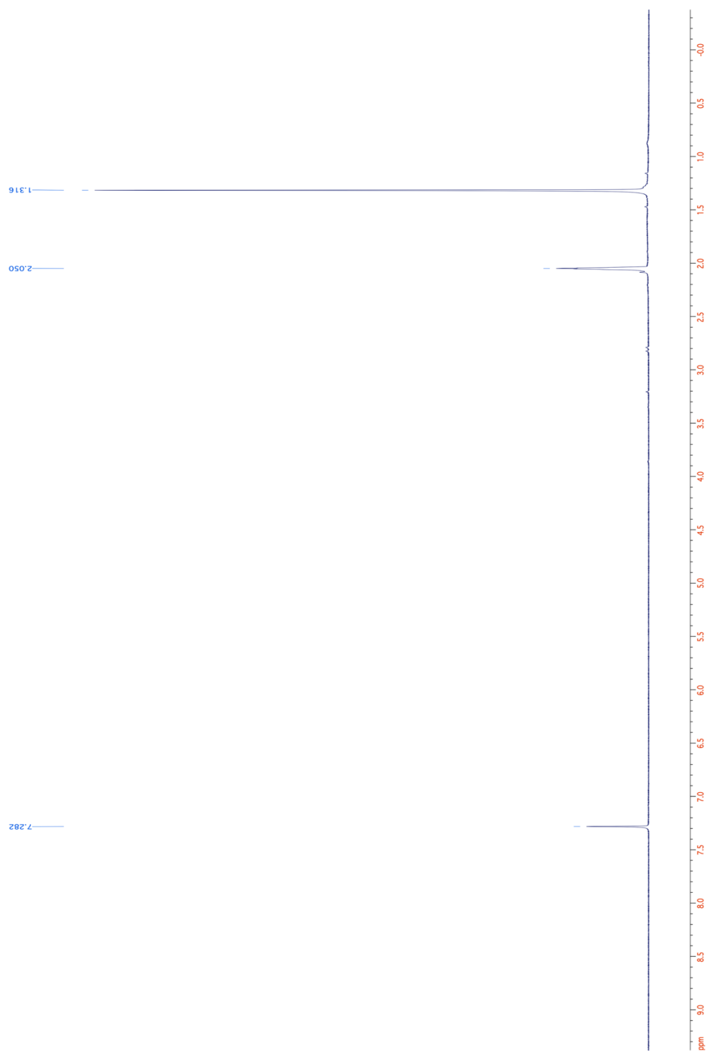
Figure 27. ^1\text{H} NMR (400 MHz, acetone- d_6 ) spectrum of crude reaction mixture of photolyzing 1,2-divinylcyclohex-1-ene ( 14 ) for 8 days.
