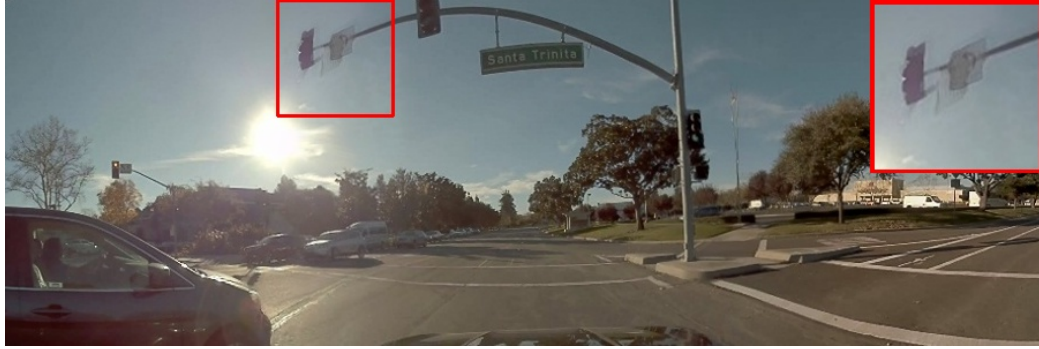
Figure 5.11: Failure case. Our approach might produce mis-alignment or ghosting artifacts when the flow estimation is not accurate enough.
