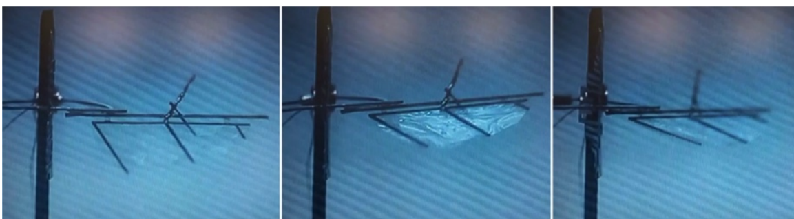
Figure 5.9: Wing pitch, front view. Wing pitch amplitude increases as the mechanism's stroke speed increases. The X-shaped CF frame hard-limits the pitch magnitude.
