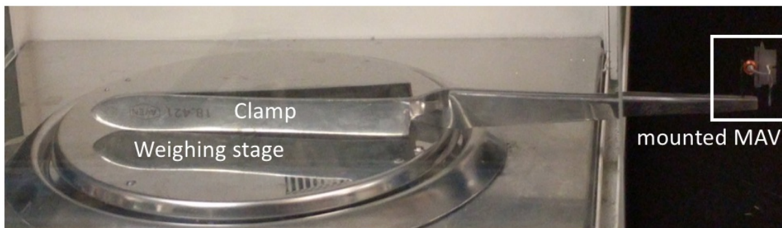
Figure 4.20: Setup for the measurement of average lift.
