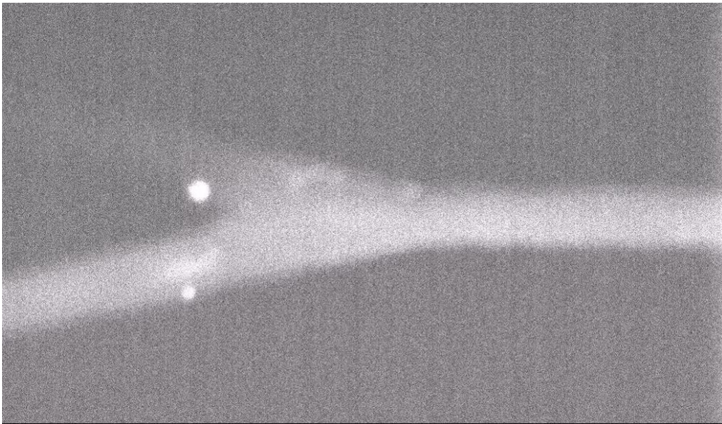
Figure 3.6 Fluorescent signal from SYTOX green at the mixing point between the red blood cell suspension and salt solution. Red blood cell suspension (bottom channel) mixes with salt solution (top channel). This image captured at 100 ms speed shows the averaged signal obtained from the channel. No red blood cells are visible using fluorescence.
