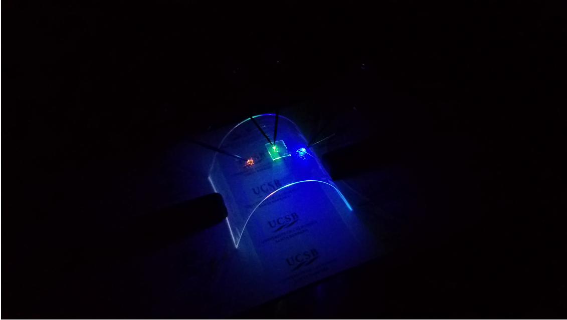
Figure 1.8: Optical photograph of red, green, and blue \mu LEDs on the same transparent and flexible substrate (acrylic) electrically lit up. The active region of the \mu LEDs were comprised of InGaN and not AlGaInP. See Chapter 5 for details of growth and fabrication.
