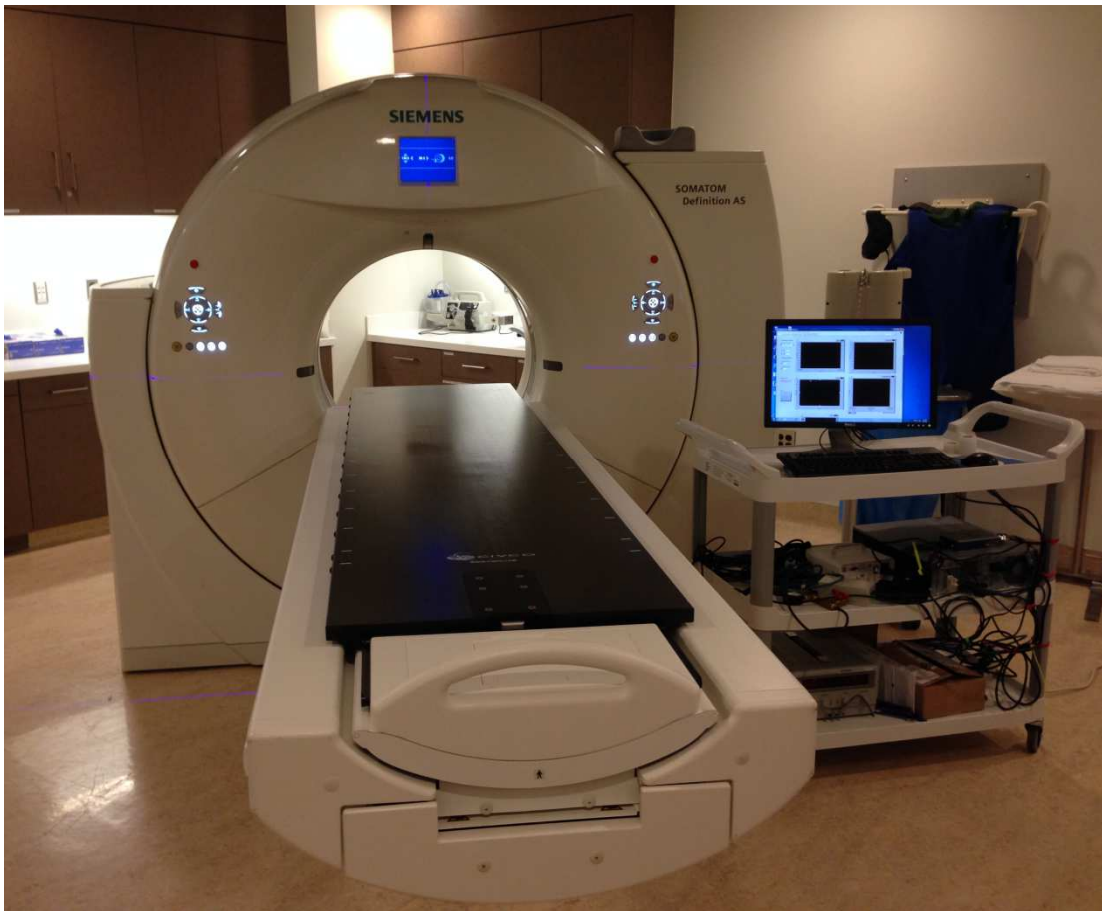
Figure 1. CT scanner and breathing signal acquisition system.
