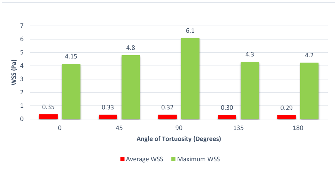
Figure 11: Bar Graph depicting the difference in the magnitudes of Maximum WSS and Average WSS with increase in angle of tortuosity of the parent vessel.
